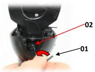
Take hold of tying head 01 and pull it to remove it from the body 02 of the machine.
