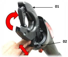
It is normal for the tying head 01 to resist and make you force it to bring it back into its operating position.
