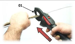
Go right up to the abutment to ensure that the arm closes fully and attaches the wire correctly.
