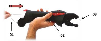
If the wire does not emerge, unclip lever 01 and pull it right out of the machine.
