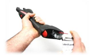
Spray directly on to the wire on the reel, once or twice per reel, to help the wire to slide more easily as it moves round the reel.
