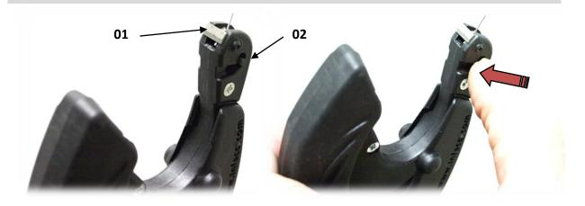
The wire may be bent at exit 01: *(no need to disconnect the machine)* simply go through the cycle empty or run the knife only and resume the tying action.
