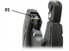
After the last tying operation it is possible that some wire may remain stuck in the tying head:
