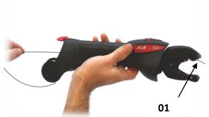
Unclip the brake system lever 01.
